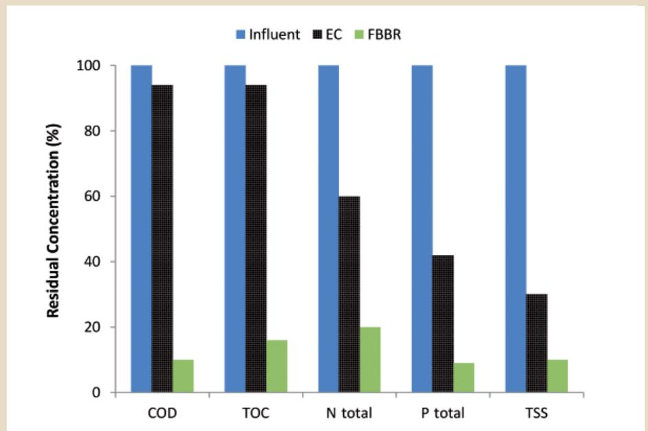
Fig. 3 Residual concentrations (%) of COD, TOC, TN, TP and TSS in wastewater after both treatment phases
