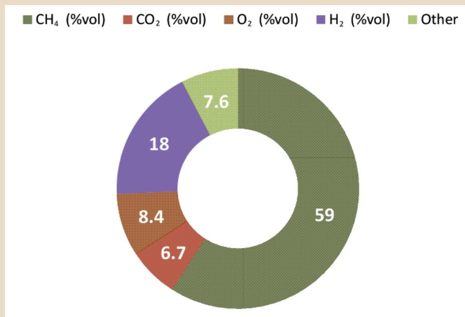
Fig. 4 Average enriched biogas composition during FBBR unit operation
