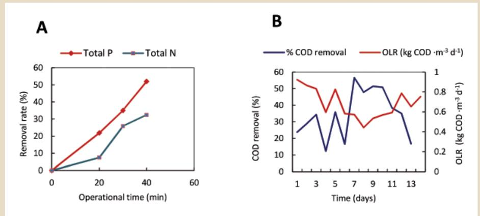
Fig. 2 A) Removal of TP and TN at a fixed current density of 2.5 mA cm<sup>-2</sup> and at different retention times in the EC; B) COD removal and organic loading rate in the FBBR
